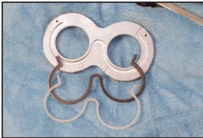
Figure 12a Pump Thrust Block - Back Side
