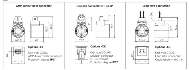
Note: For the electric characteristics refer to standard coils features - see section 3
