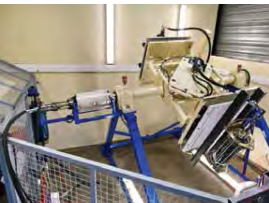
Accumulator test bench for wind turbine application.
